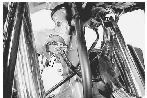
**“C44” HO2 SENSOR (HO2S) CIRCUIT MALFUNCTION (E-02, 19)**
