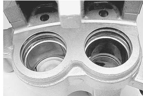
Inspect the brake fluid leakage from O-ring ① and cup ②. If any abnormal condition found, replace the rear brake caliper.
